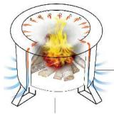
Secondary air supply rises through double outer walls and exits holes at top of pit
